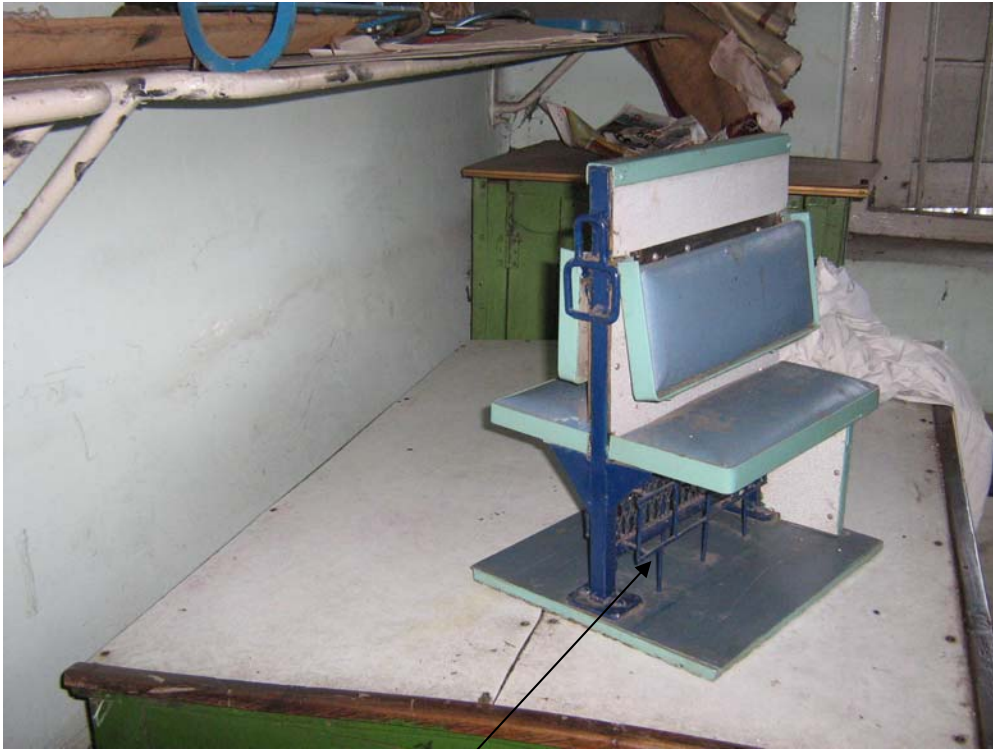
A cut model of coach berth showing the location of 'Wire Screen' Wire Screen
